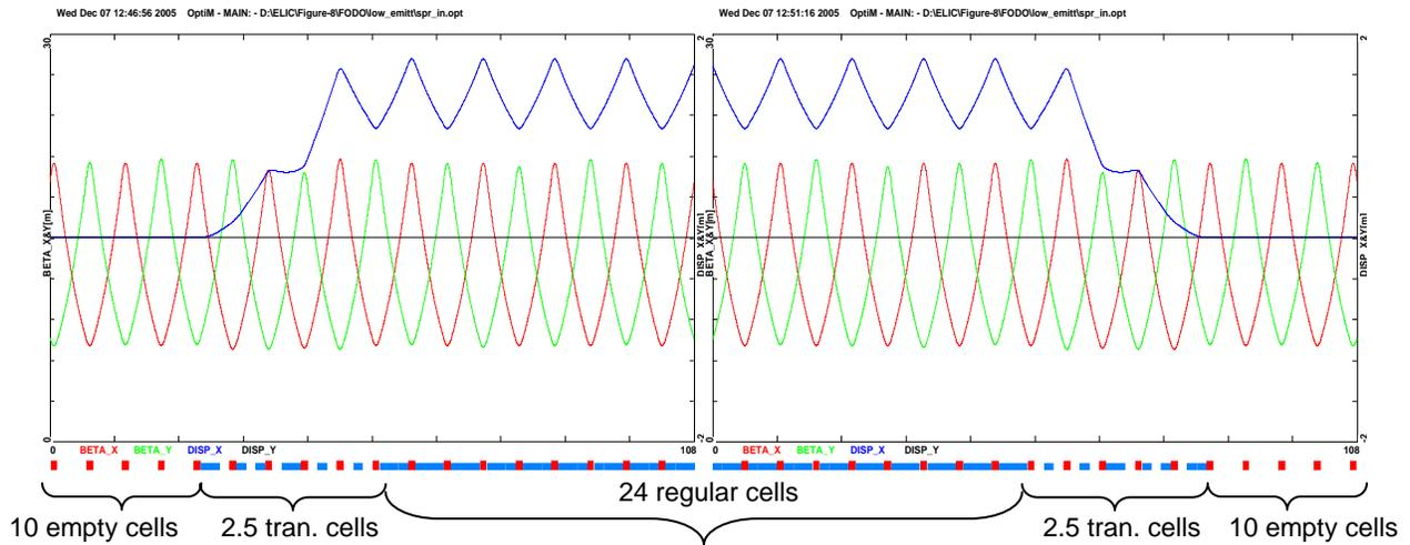
Figure 4 Linear optics at 150 GeV for one half of the Figure-8 ring with 60 deg. crossing.
