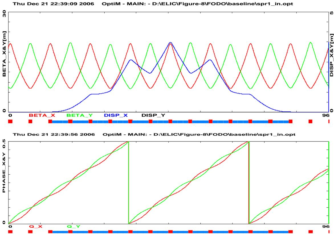
Figure 2 Achromat super-period – Twiss functions (top) and betatron phase advance in units of  $2\pi$  (bottom)
