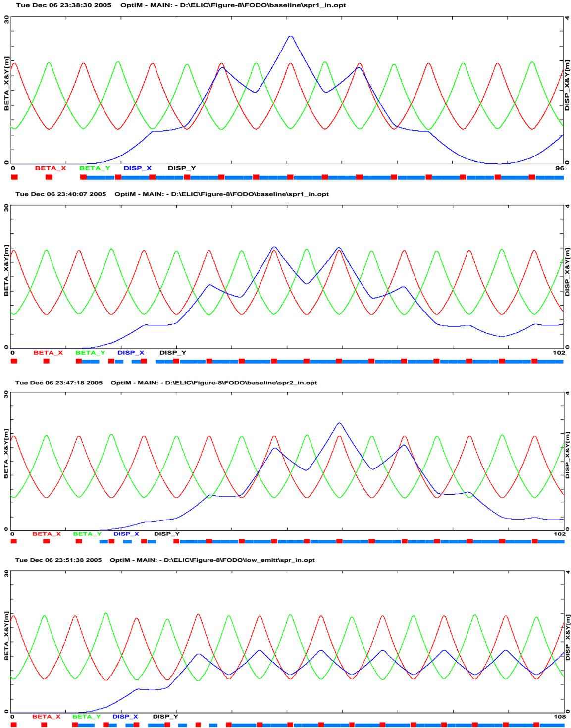
Figure 3 Minimizing the average dispersion in the ring by removing specific dipoles from the transition cells.
