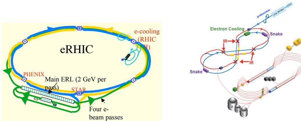
**FIGURE 1.** Two possible design layouts of the Electron Ion Collider project. Left panel: [eRHIC] the EIC version at RHIC is shown. Right panel: [ELIC] is the corresponding version at JLab .
