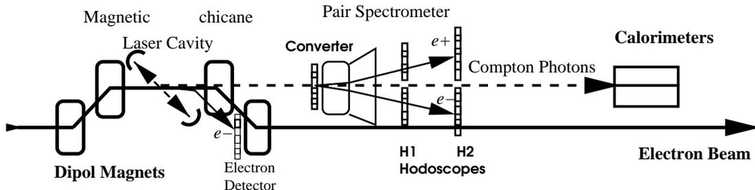
FIGURE 4. Schematic view of a possible Compton polarimeter for the EIC.
